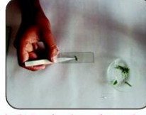
(g) Taking the thin section with brush
