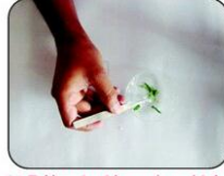
(g) Taking the thin section with brush
